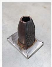
Combustion Chamber SS316L – Aerospace
