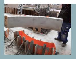
3D printed patterns and molds can replace expensive CNC milled or hand-crafted traditional forms. By modernizing the first phases of numerous casting applications, the BigRep ONE allows you to produce in-house, iterate faster, cut material costs, and streamline logistics. BigRep customers use the ONE to print forms for making carbonfiber parts like drones and custom auto bodies, for various kinds of concrete casting, and to produce patterns for anything from bathtubs to propellers.
